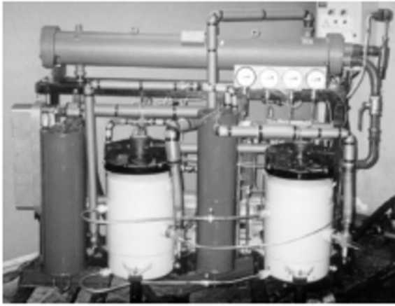
Fig. 13. Pilot-production vapor-compression heat pump for obtaining hot water in heating systems with simultaneous production of cold.
