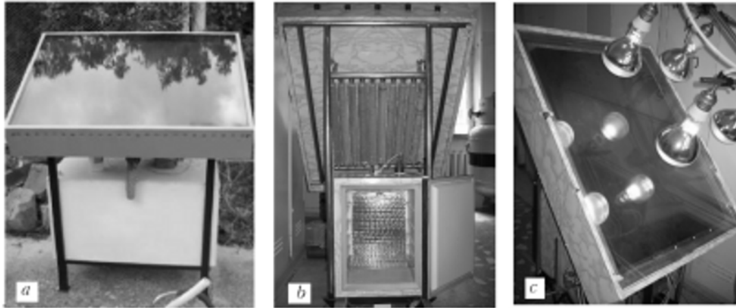
Fig. 15. Solar adsorption coolers according to [59] (a) and [60] [b] refrigerating chamber and condenser, c) heating by electric lamps].
